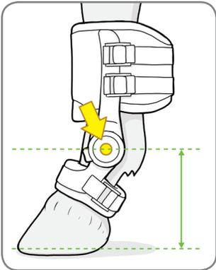
8. Check that the center of the SafeStop™ is at the same height off the ground as the Center of Rotation, i.e. the 2 axes of rotation should be in alignment.
