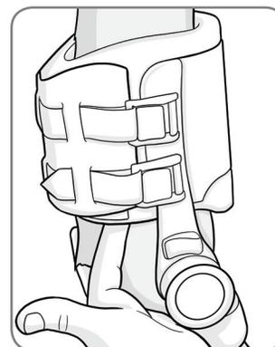
5. Check the fit of FastTrack™ to ensure the padding has formed correctly to the horse's leg. The heating process may be repeated to achieve a better fit if necessary.
