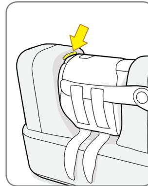
4. You should be able to fully see both padding alignment marks when FastTrack™ is properly installed.
