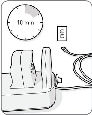
1. Unplug Heater Kit. Allow device to cool down for 10 minutes or as needed.
