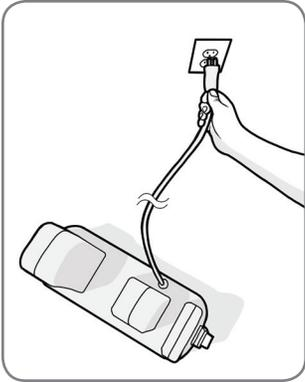
6. Uncoil power cord fully and plug into standard 120 VAC outlet. Cord should not cross over the top surface of the Heater Kit in any way.
